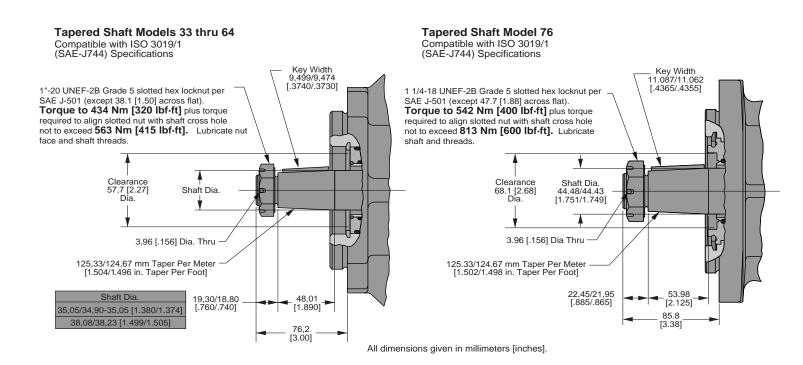
Heavy Duty Series Tapered Shaft Torque – Specifications
