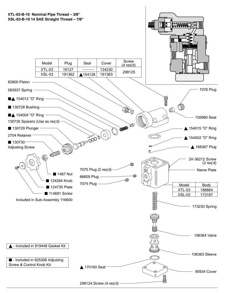
For satisfactory service life of these components, use full flow filtration to provide fluid which meets ISO cleanliness code 18/15 or cleaner. Selections from Eaton OFP,OFR and OFRS filter series are recommended.
